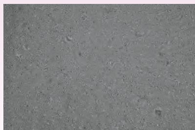
Surface of Imprint™ 4 Preliminary VPS Material shown with a Laser Scanning Microscope (objective lens with 20x magnification).
